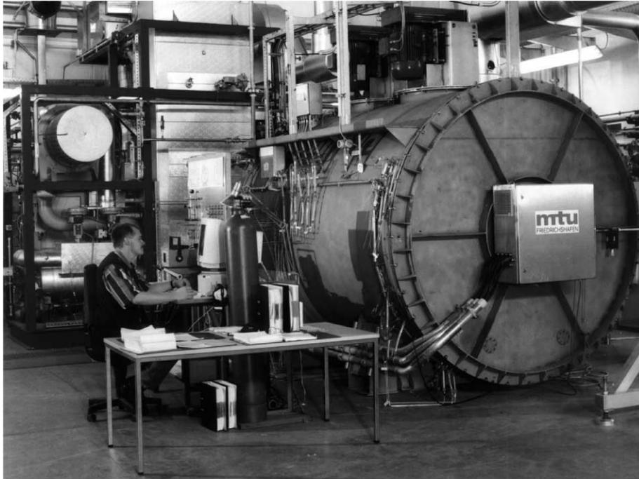
Fig. 7. The Hot Module during test at the Ruhrgas test facility, Dorsten, Germany.
