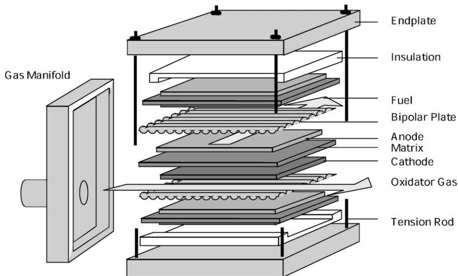
Fig. 4. Structure of a cross-flow fuel cell stack.
