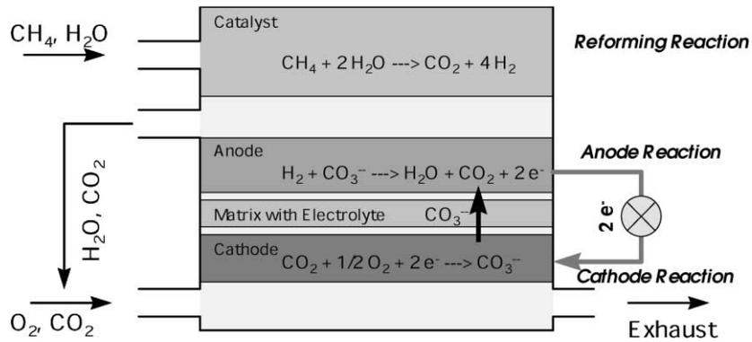
Fig. 2. Operating principle of molten carbonate fuel cell with internal reforming.
