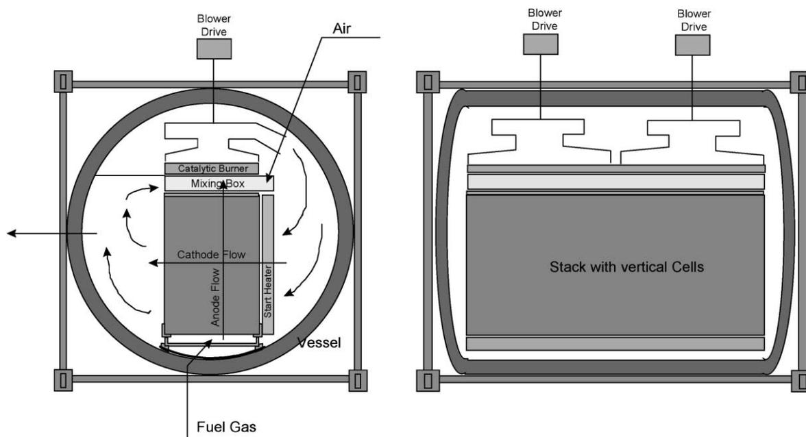
Fig. 5. Basic design of the Hot Module.
