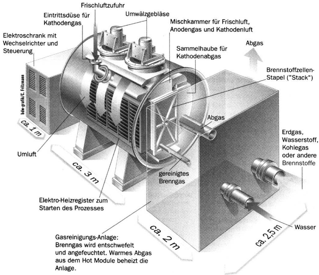
Fig. 6. Direct fuel cell cogeneration Hot Module prototype.
