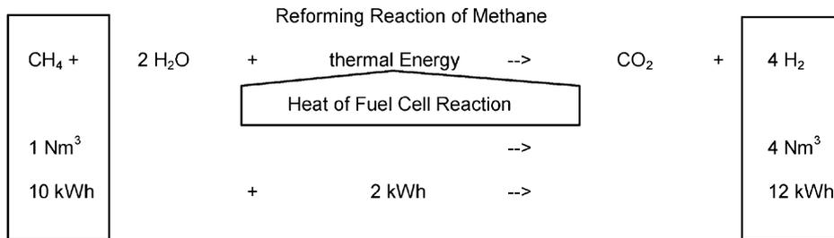
Fig. 3. Increase in efficiency of high temperature fuel cells by internal reforming (2 kW h primary energy production from “waste” heat and 12% gain of efficiency at 60% fuel utilization).
